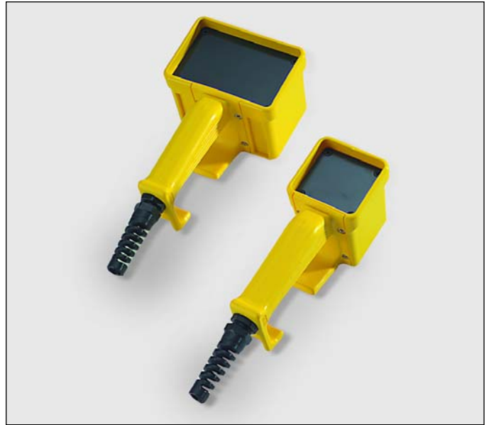
Control Units 2930 (left) and 2940: Each enclosure consists of a one-piece glass-filled polyamide enclosure body, polyester round-cornered front panel with screws, stamped foam rubber gasket, wall-mount bracket, and M20 cable grip. Power cord cable grips are designed to offer bending protection and strain relief.
