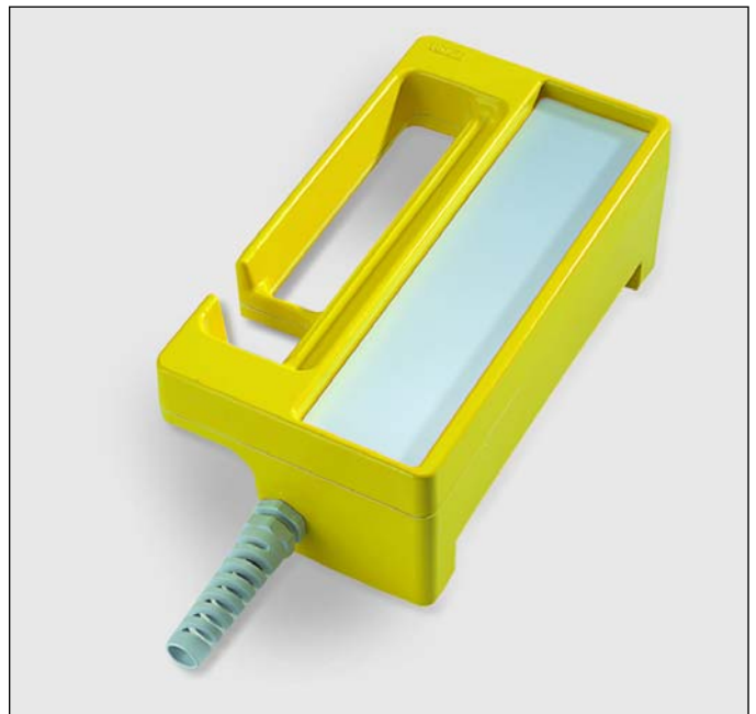
Control Units 2950: Each enclosure consists of a reinforced fiber-glass enclosure lid and base, self-adhesive bright anodized aluminum front plate, round Neoprene gasket, wall-mount brackets, and M25 cable grip. Power cord cable grips are designed to offer bending protection and strain relief.
